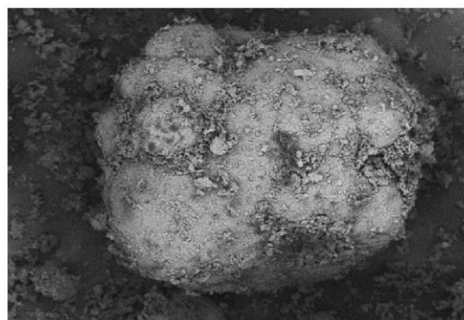
Fig. 4. (a–b) Nucleation, coating and coalescence between nuclei (Regime I), size class ( 160\text{--}250 \mu\text{m} ), L/S=31.7\% , top = 19 min, N=500 rpm.
