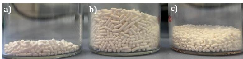
Figure 16. Pellets obtained from formulations a) 8, b) 7 and c) 5 after calcination at 500°C.
