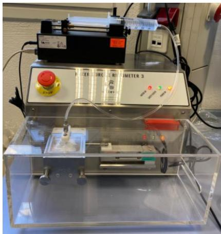
Figure 10. Caleva Mixer Torque Reometer
